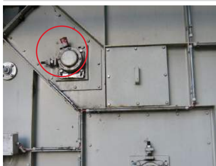
Lubrication of flange bearing on bucket conveyor
